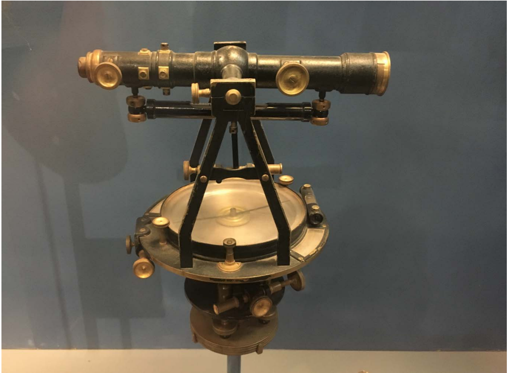
Surveying transit made by W. & L. Gurley, Troy, NY, used to survey ranches in the Texas Panhandle in the late 19 th century. Panhandle Plains Historical Museum, Canyon, TX.
